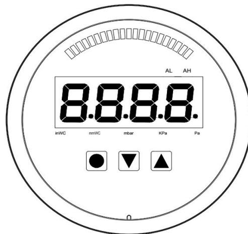
○ key is the setting key, △ is used to set the unit (Pa->KPa->mbar->mmWC->inWC->Pa) in the reality interface, ▽ key is used to clear the zero. See item 4.3 for specific use.
