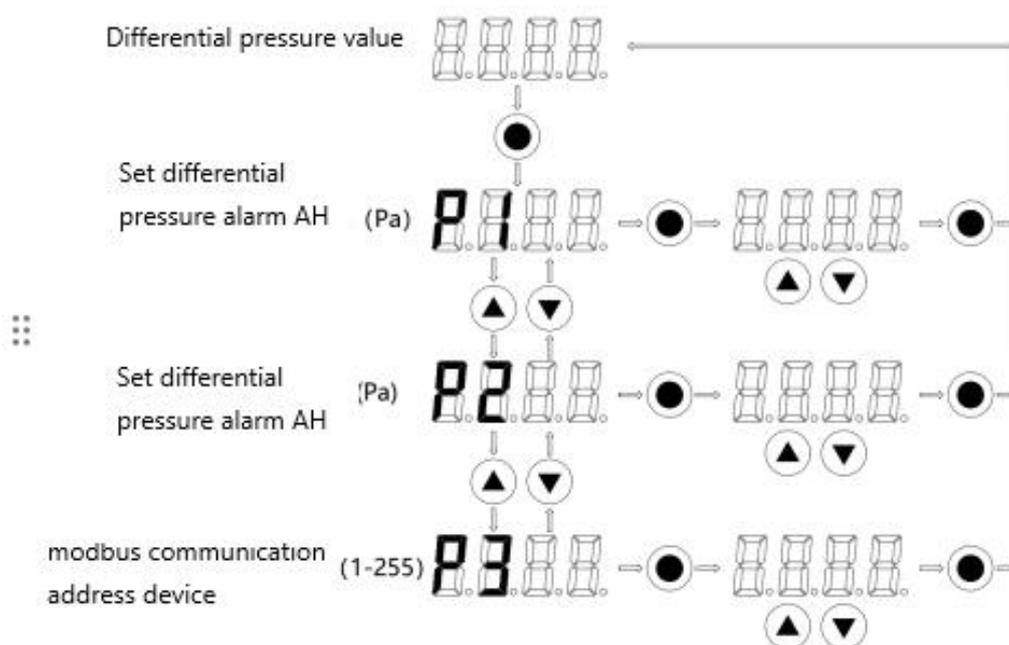
Press  $\circ$  setting key to enter the setting interface, use  $\Delta$  and  $\nabla$  keys to adjust the setting items, every time you press  $\Delta$  plus 1, every time you press  $\nabla$  minus 1, press and hold for fast plus or minus.
